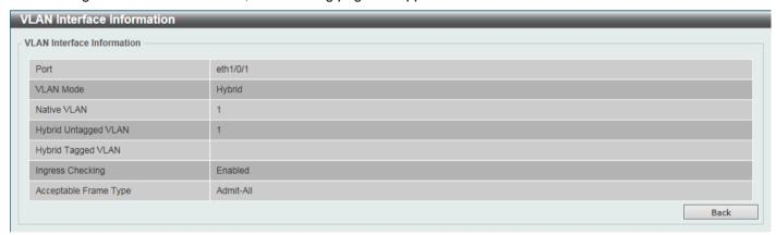
Figure 5-14 VLAN Interface (VLAN Detail) Window
