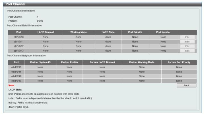
Figure 5-43 Link Aggregation (Channel 1 Detail) Window
