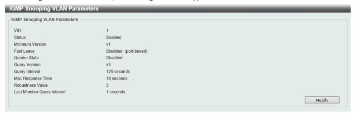
Figure 5-47 IGMP Snooping Settings (Show Detail) Window
