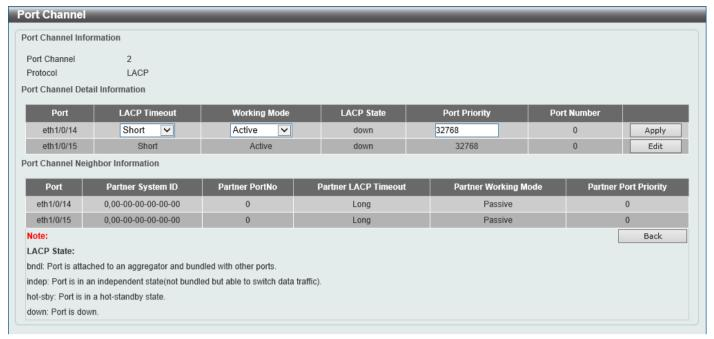
Figure 5-45 Link Aggregation (Channel 2 Detail, Edit) Window
