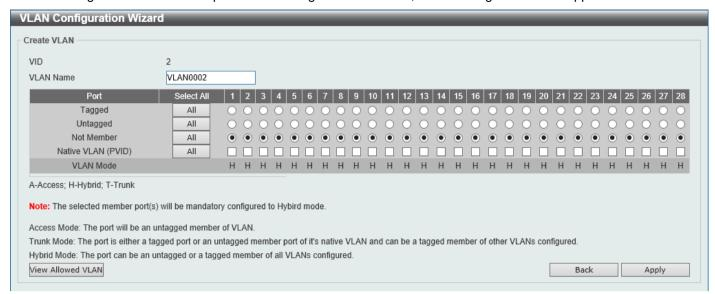
Figure 5-8 VLAN Configuration Wizard (Create VLAN) Window
