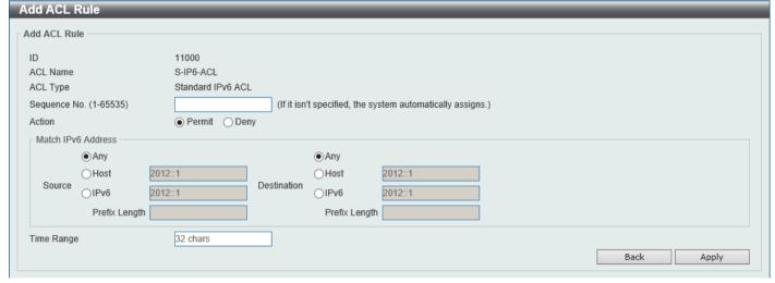
Figure 8-13 Standard IPv6 ACL (Add Rule) Window
