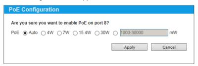
Figure 14-2 PoE Configuration (To Enable) Window
