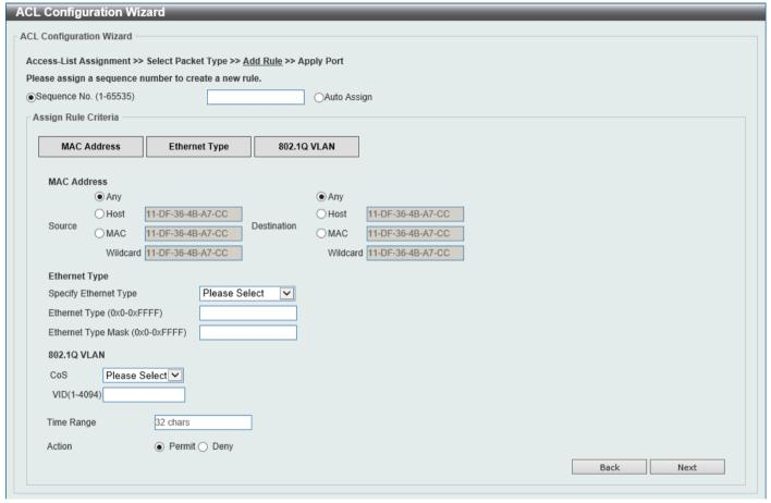
Figure 8-4 ACL Configuration Wizard (Create, Packet Type, MAC) Window
