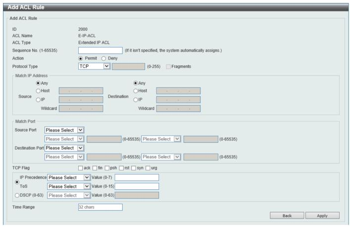
Figure 8-12 Extended IP ACL (Add Rule) Window
