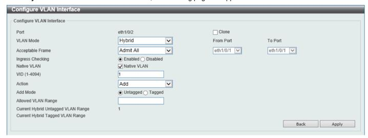
Figure 5-16 VLAN Interface (Hybrid) Window
