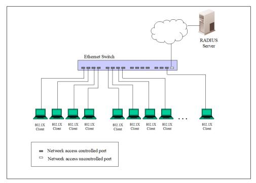
Figure 9-10 Example of Typical Port-based Configuration
