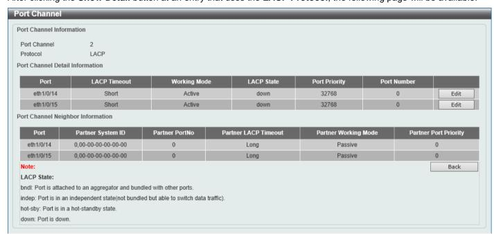
Figure 5-44 Link Aggregation (Channel 2 Detail) Window
