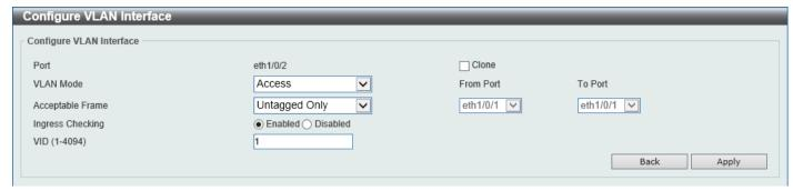
Figure 5-15 VLAN Interface (Access) Window
